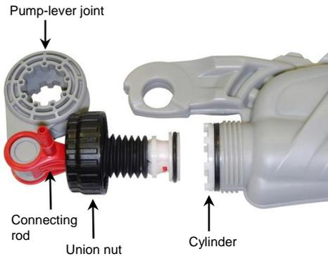
Loosen the union nut and pull the pump-lever Joint, together with the connecting rod and the piston, out of the cylinder. Remove the pump-lever joint. Turn the connecting rod and piston unit 180° and mount the pump-lever joint again.
