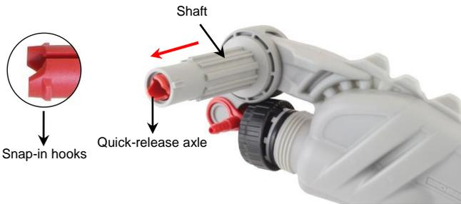
Press the snap-in hooks together and pull the shaft out from the quick-release axle.
