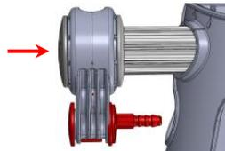
Move the pump lever into the assembly position (approx. 45° angle), note the shaft markings (cams on the front and ridge without an indentation) and insert until it locks into position (first latch, adjustment position).
