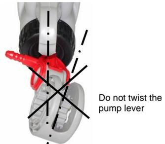
Carefully insert the whole unit into the cylinder in the pump handle. Align pump-lever joint to the pump lever (do not twist). Push the connecting rod in and tighten the union nut. Mount the shaft and quick-release axle (see guidance image).
