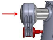
Turn the pump lever in the desired position as far as it will go (working or parking position) and insert fully until it has completely locked into position (second latch, function position).
